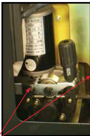
(9) Fit the correct sized Knurled Drive roller for Gas Less Flux Cored wire
