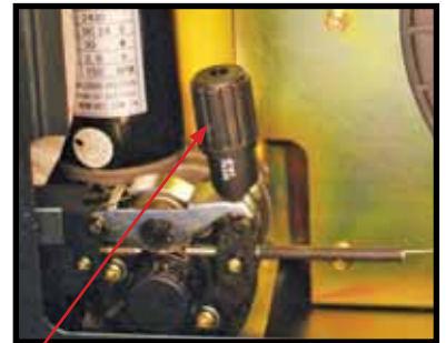
(13) Apply a medium amount of pressure to the drive roller
