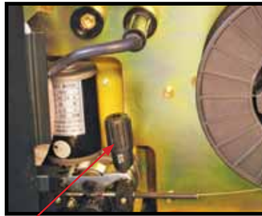
(13) Apply a medium amount of pressure to the drive roller
