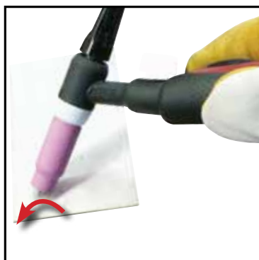
(12) With a small movement rotate the Gas Cup forward so that the Tungsten Electrode touches the work piece.
