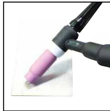
(11) Lay the outside edge of the Gas Cup on the work piece with the Tungsten Electrode 1- 2mm from the work piece.
