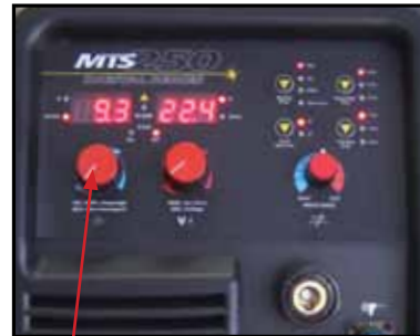
(9) Set the welding current using the amperage control dial
