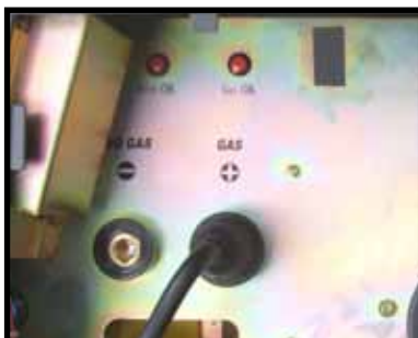
(9) Connect weld power lead to GAS ⊕
