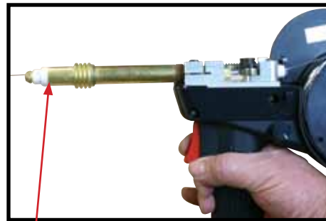
(16) Remove the gas nozzle and contact tip. Pull the trigger to drive the wire through the neck until it exits the contact tip holder
