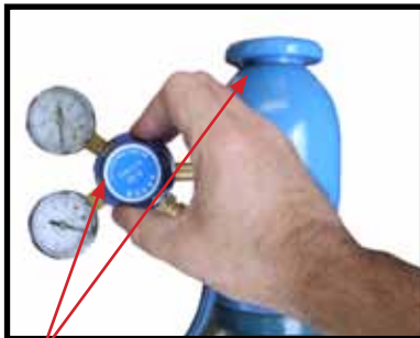
(8) Carefully open the valve of the gas cylinder, set the flow to 6-10 l/min
