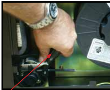
(12) Close down the top roller bracket and clip the pressure arm into place.
