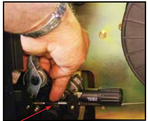
(11) Feed wire over the drive roller into the outlet guide tube, Push the wire through approx 150mm.
