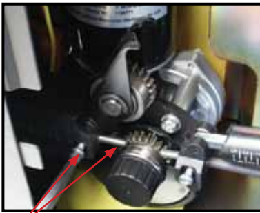
(10) Loosen the inlet guide tube retaining screw.
